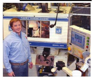
He added that the toolmaker only removes a small crosssection of material when grinding microdrills, and that wear on the grinding wheel is negligible. "It's not the same as huge stock removal--- we probably damage more wheels than we use up".
