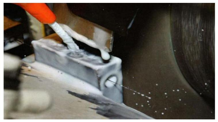
M&S hold tolerance down to 0.00002" on ground parts. Shown is a secondary diameter of 0.010" being ground on a cardiac guide wire.
