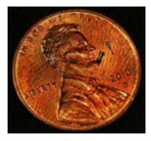
Two examples of the tiny parts ground at M&S are a 0.058" long barbellshaped locking pin for a heart valve repair device and an H13 tool-steel core pin for a medical product mold which is 0.090" long with diameters of 0.003" and 0.012".
